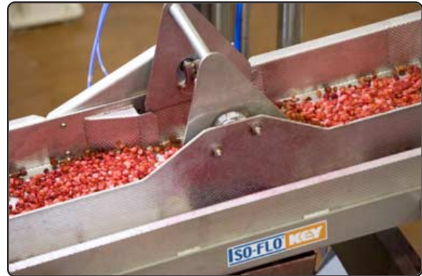
This Iso-Flo vibratory shaker incorporates a swing gate for distribution of in-process Craisins.
