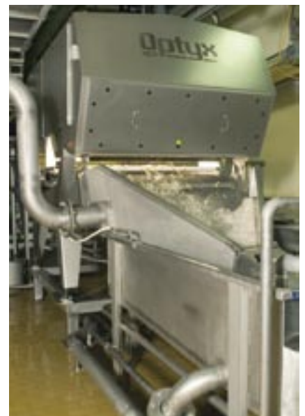
Discharge from Optyx on potato strip line
