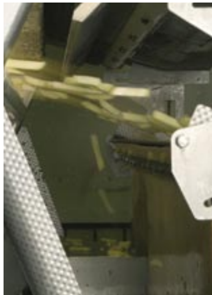
Optyx ejector system on potato strip line
